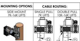
MOUNT HARDWARE: 5/8" STAINLESS STEEL \*THRU BOLTED\* LENGTH DETERMINED BY
