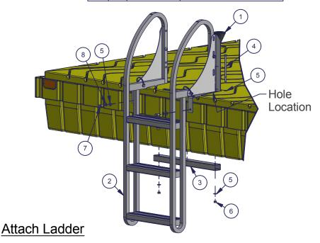
Step 1. The rear of each Ladder Pivot is bolted through the hole marked on the drawing as Hole Location. Two 3/8" x 6-1/2" bolts and two 3/8" washers are placed through the rear of each ladder pivot. The bottoms of the two bolts are secured through a Ladder Brace using two 3/8" washers and two 3/8" Nyloc nuts.
