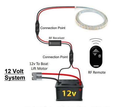
Warning: Only connect the RF Receiver to ONE 12v Battery
