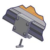
Pivot the top lip of the Accessory Connectory Bracket assemby into the Groove on the top of the dock frame - as shown.
