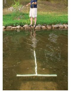
**To attach the filament**, thread through the holes found at the tips of the rake teeth. Tie the filament at each end tooth using a fisherman's improved clinch knot.
