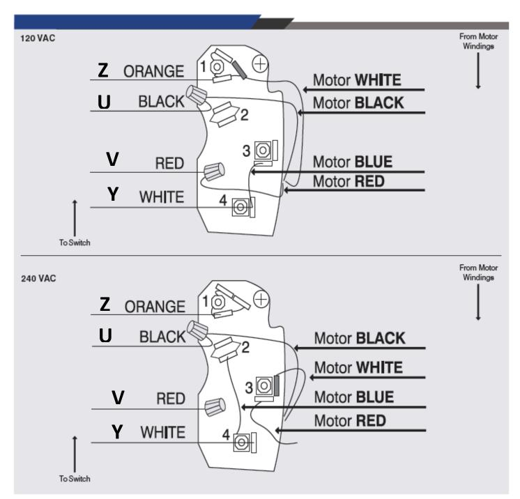
To change motor direction, switch Orange & White Controller wires.
