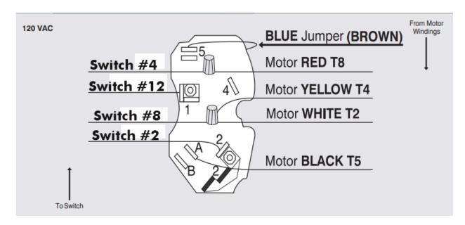
**Note:** Wire color is not standard between different manufacturers. To make sure the motor is wired correctly, please use the switch and motor terminal numbers and not the colors.
