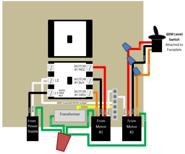
Use the diagram below if your motor is a new 56 frame Aqua Marine Supply motor from Regal Beloit
