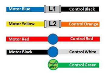
Use the diagram below if your motor is a 56 frame Aqua Marine Supply motor from Regal Beloit/AO Smith with terminal board
