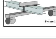
The dual pipe support for steel mounting (Picture 1) is specifically designed to line up with the BHUSA hoist hanger (Picture 2) and will not work unless used with the steel hoist hanger.
