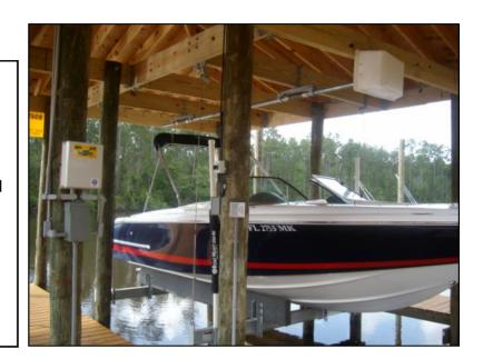
Mount the Boat Hoist USA hoist to the joist that will not be supporting the blocks. The hoist and pipe supports should be mounted in the center of the slip. See Figure 1. Use only two holes (not all four) to mount the hoist to the joist.
