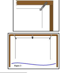
The dual pipe supports are designed to mount in the center directly under a joist. This will allow the cable to line up with the blocks.
