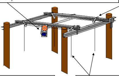
Angle the galvanized I-beam clamps (Picture 3) towards the boat at a 45 degree angle. This will eliminate unnecessary torque and help the clamps from sliding on the I-beams while being used on extreme loads. Clamps can be used on I-beams, channels or Tubing.
