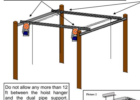
Each lifting point will require its own length of cable. Find the center of each dual pipe support and drill a hole in one side of the pipe. Run the end of the cable through the hole, and then feed it through the shaft of the pipe and out the end. Attach a cable clamp, and then pull the cable back through pipe.
