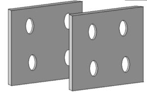
There are three tabs welded to the main drive pipe and one tab welded to the dock mount and one tab welded to the included pile mount clamp. The tabs bolt together to support the drive pipe on the dock
