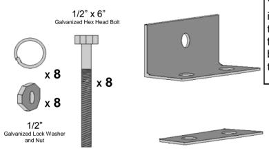
Your lift is supplied with 4 x pc of angle and 4 x backing plates. These will for your bunk brackets. Install these brackets on the square tubing at the bottom of the main ride carriage using 2 x 1/2" x 6" Hex Head bolts for each bracket. Sandwich the bracket to the tubing using the flat back up plate.
