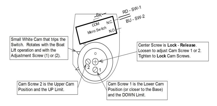
Tools required: Phillips Head screwdriver, Small Slotted Head Screwdriver,
