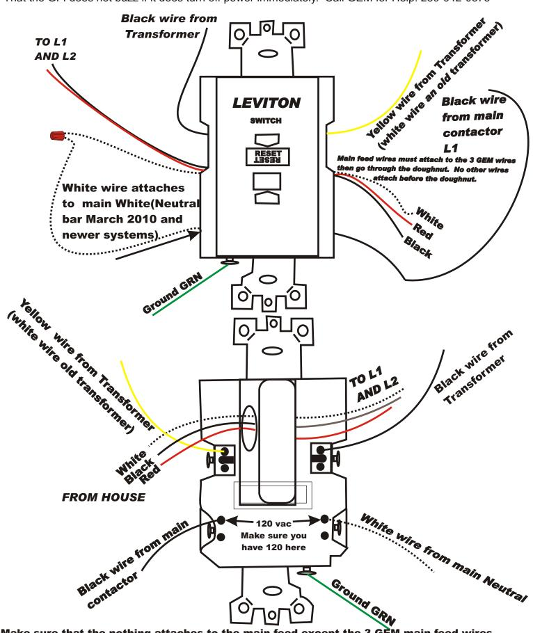
Make sure that the nothing attaches to the main feed except the 3 GEM main feed wires (Red, Black and White)they must go trough the doughnut then you may split off main feed wires.
