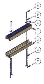
NOTICE Check pile guide for a 1/8" hole 7/16" from the top centered on the side that mates to the dock section. Be sure the guide is oriented so the hole is above the water if applicable.
